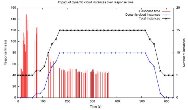
Figure 4: Impact of dynamically adding cloud instances over response time
